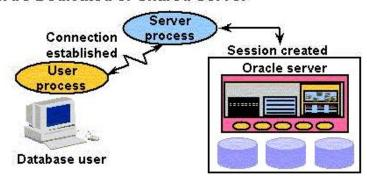
A Server Process is the go-between for a Client Process and the Oracle Instance.
